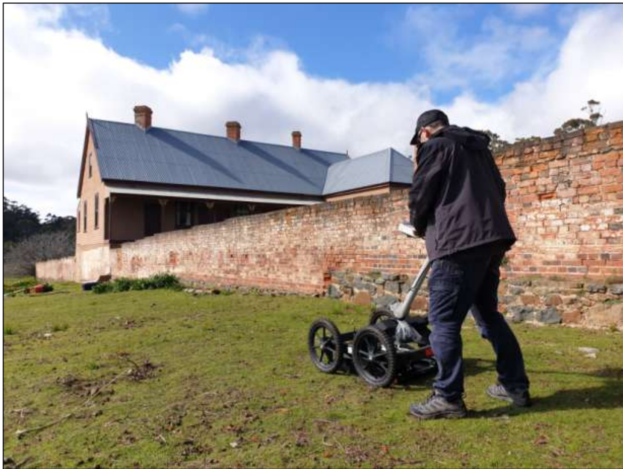
Ground Penetrating Radar
